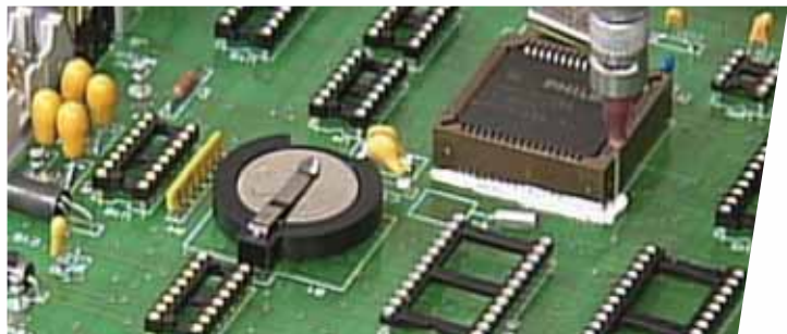
The SCS Precisioncoat RTV applies a fine line around delicate components.
