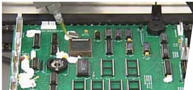
The SCS Precisioncoat RTV offers continuous, motor-driven tilt and rotate application.
