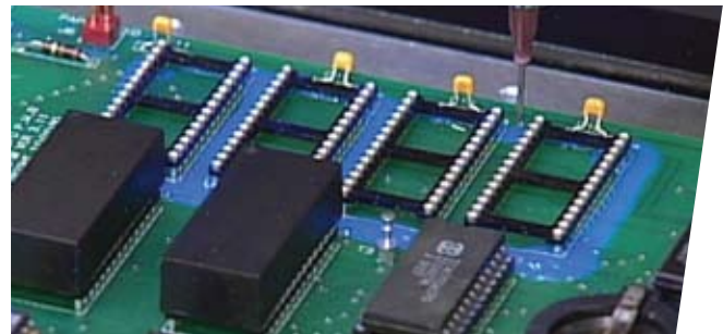
The SCS Precisioncoat is mechanically accurate to 0.001 inches.
